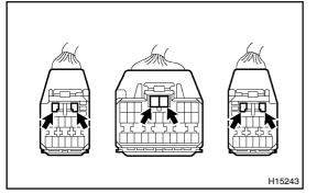
OK: No deformation is identified. HINT: Compare it with the other 2 connector pins.
