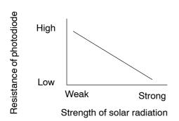
A photo diode in the solar sensor detects solar radiation and sends signals to the A/C amplifier.
