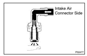
(b) Blow air into the intake air connector side, and check that air passes through with difficulty.
