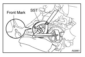
(c) Holding the hexagon portion of the camshaft with a wrench.
