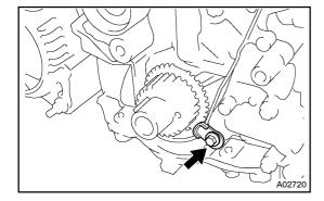
(c) Install the timing belt plate with the bolt.
