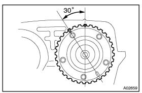
(b) Check that the outer circumference of the VVT-i pulley easily rotates through 30°.
