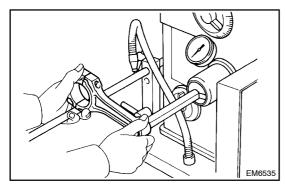
(d) Using a pin hole grinder, bore the bushing to obtain the standard specified clearance (See page EM-85) between the bushing and piston pin.
