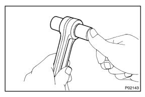
(e) Check the piston pin fit at room temperature.
