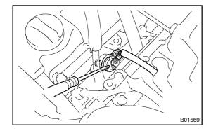
(2) If you have no sound scope, you can check the injector transmission operation with a screwdriver.
