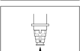
(n) Connect SST (wire) to the injector and battery for 15 seconds, and measure the injection volume with a graduated cylinder. Test each injector 2 or 3 times.
