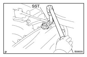
(c) Using SST, remove the pulsation damper and 2 gaskets. SST 09612–24014 (09617–24011)
