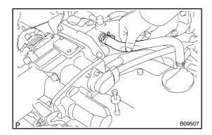
(3) With engine idling, pinch the air assist hose and check that engine speed drops, and then returns back up to idle speed.
