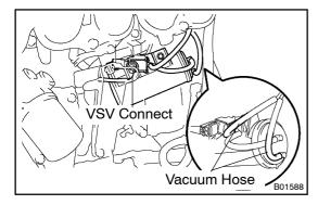
(b) Disconnect VSV connector and vacuum hoses, and remove the vacuum control valve set.
