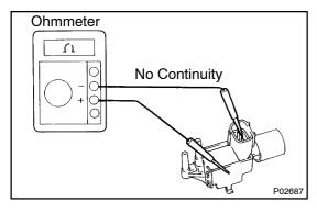
(b) Inspect the VSV for ground.Using an ohmmeter, check that there is no continuity between each terminal and the body.
