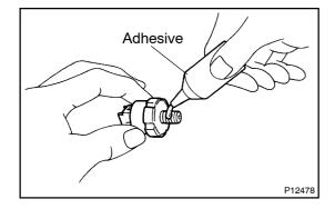
(h) Apply adhesive to 2 or 3 threads of the oil pressure switch.
