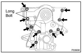
(d) Install the oil pump with the 9 bolts. Torque: 21 N·m (210 kgf·cm, 15 ft·lbf)
