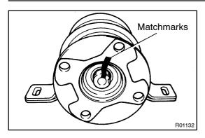
(k) Align the matchmarks on the universal joint flange and intermediate shaft, and install the universal joint flange.
