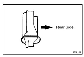
(i) Install a new center support bearing to intermediate shaft. HINT:
