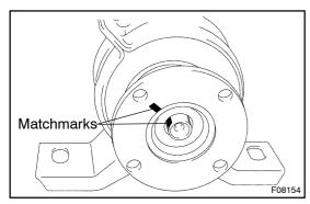
(e) Place matchmarks on the universal joint flange and intermediate shaft.
