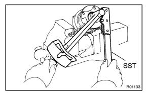
(m) Using SST to hold the flange, install a new nut. SST 09330-00021
