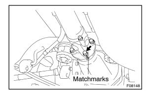
(d) Align the matchmarks and install the propeller shaft on the differential with the 4 bolts, washers and nuts.
