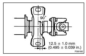
(e) Torque the 2 center support bearing set bolts.
