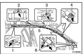
(d) In the order shown in the illustration, remove the bolts and curtain shield airbag assembly.
