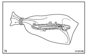
(e) Put the removed curtain shield airbag assembly into a clear plastic bag and keep it in a safe place.
