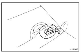
(b) Put the removed curtain shield airbag assembly into a clear plastic bag and put it on the instrument panel.
