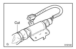
(b) Cut off the deployment section in airbag from inflator.
