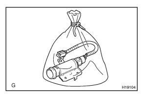
(h) Dispose of the curtain shield airbag assembly.
