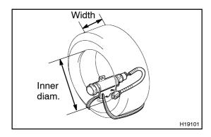
Position the curtain shield airbag assembly inside the tire with the airbag deployment direction facing inside.
