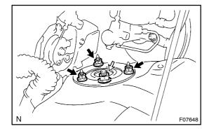
(c) Loosen the nut in the center of the suspension support.
