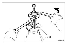
(c) Using SST, remove the companion flange. SST 09950-30012 (09951-03010, 09953-03010, 09954-03010, 09955-03030, 09956-03020)
