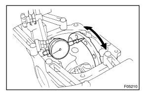
(f) Using a dial indicator, while turning the companion flange measure the differential case runout.
