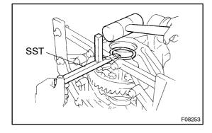
(c) Using SST and a plastic hammer, remove the 2 plate washers.
