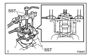
(c) Torque sensing LSD ring gear back side: Using SST, remove the side bearing from the differential case.
