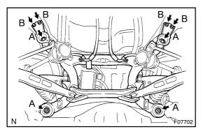
(b) Install the 2 differential support member lower stopper, rear suspension member stopper with the 8 bolts.
