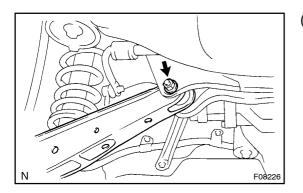
(e) Remove the nut, washer, bolt and No. 2 lower suspension arm from the rear suspension member.
