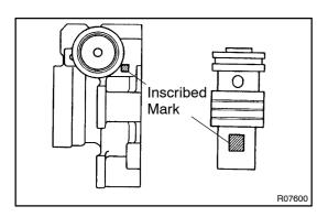
If necessary, replace the flow control valve with one having the same letter as inscribed on the front housing.
