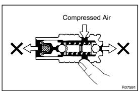
(b) Check the flow control valve for leakage.
