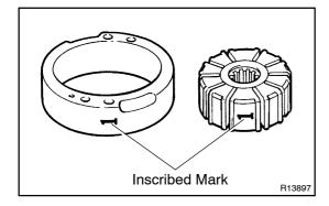
If it is more than the maximum, replace the vane plate and/or vane pump rotor with one having the same mark stamped on the cam ring.
