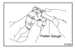
(b) Using a feeler gauge, measure the clearance between the vane pump rotor groove and vane plate.
