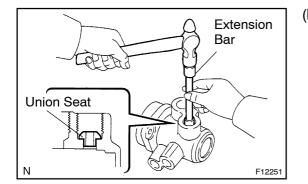
(b) Using a plastic hammer and extension bar, lightly tap in a new union seat.
