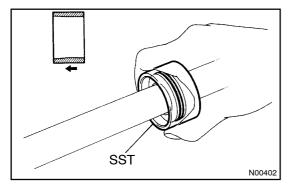
(f) Carefully slide the tapered end of SST over the teflon ring until it fits to the steering rack.
