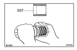
(e) Carefully slide the tapered end of SST over the teflon rings until they fit to the control valve assembly.
