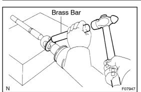
(c) Using a brass bar and a hammer, stake the washer. **NOTICE:**
