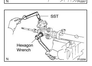
(f) Using SST, a torque wrench and hexagon wrench (24 mm), tighten the rack guide spring cap until the preload is within the specification.
