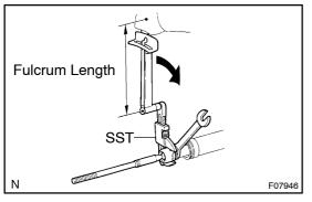
(b) Using a spanner, hold the steering rack steadily and using SST, torque the rack end.
