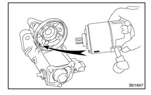
(c) Pull out the field frame together with the armature.
