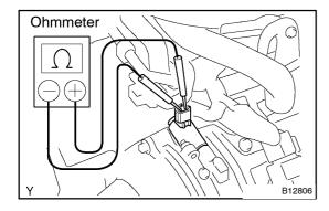
(d) Using an Ohmmeter, measure the resistance between the terminals.
