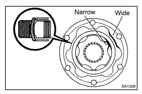
(a) Align the matchmarks placed before removal.
