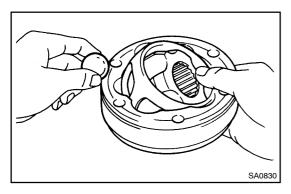
(b) Tilt the cage and inner race to the side and insert the balls one by one.
