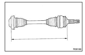
(e) The drive shaft is designed to move  $\pm 20$  mm (0.79 in.) from the normal position.
