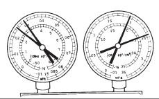
NOTE: These gauge indications occur when the refrigeration system opens and the refrigerant is charged without vacuum purging.
