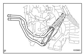
(b) Install the bracket with the screw.
