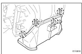
(b) Release the 4 claws and remove the air duct sub-assembly.
