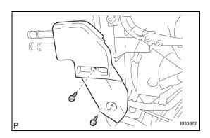
(c) Install the piping cover with the 2 screws.
