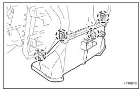
(e) Install the air duct sub-assembly with the 4 claws.
