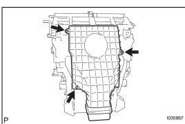
(f) Install the air duct sub-assembly with the 3 screws.
