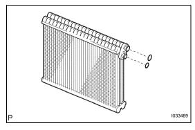
(e) Remove the 2 O-rings from the cooler evaporator No. 1 sub-assembly.
