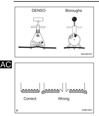
(b) Using a belt tension gauge, check the V belt tension.
