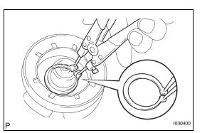
(g) Using a snap ring expander, remove the snap ring and magnet clutch stator.
