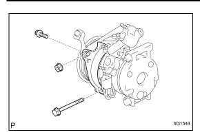
(c) Remove the 2 bolts, nut and the cooler compressor bracket.
