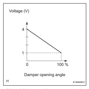
This sensor detects the position of the air inlet control servo motor and sends the appropriate signals to the A/C amplifier assembly. The position sensor is built in the air inlet control servo motor.
