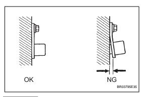
(a) Check the speed sensor installation.
