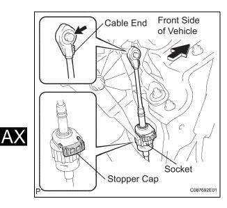
(e) Remove the 3 bolts and disconnect the transmission control cable assembly from the vehicle.
