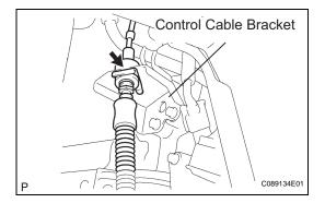
(c) Remove the clip and disconnect the transmission control cable assembly from the control cable bracket.
