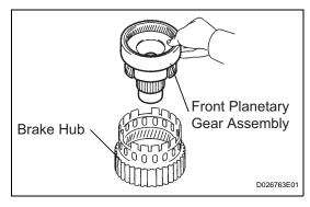
(d) Remove the front planetary gear assembly from the brake hub.
