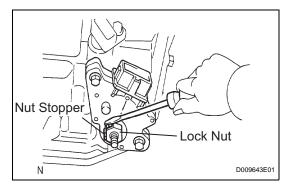
(b) Using a screwdriver, unstake the nut stopper, and remove the lock nut and nut stopper.
