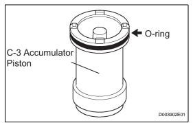
(c) Remove the O-ring from the C-3 accumulator piston.
