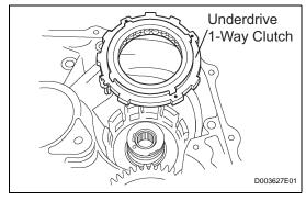
(b) Remove the underdrive 1-way clutch from the transaxle case.
