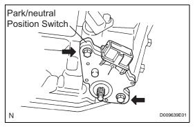
(c) Remove the 2 bolts and pull out the park/neutral position switch.
