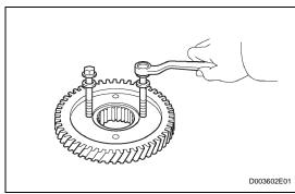
(b) As shown in the illustration, tighten the 2 bolts evenly and make clearance of approx. 20.0 mm (0.787 in.) between the counter drive gear and the inner race.
