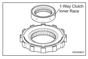
(b) Remove the 1-way clutch inner race from the 1-way clutch assembly.
