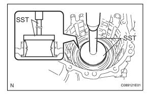
(b) Using SST and a press, remove the bearing outer race.
