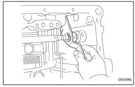
(c) Remove the manual valve lever shaft and manual valve lever.
