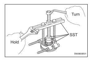
(c) Using SST, remove the tapered roller bearing.
