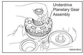
(d) Remove the underdrive planetary gear assembly from the transaxle case.
