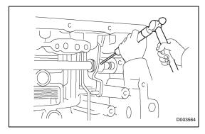
(b) Using a pin punch ( $\phi$ 35 mm) and hammer, drive out the pin.
