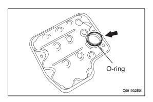
(b) Remove the O-ring from the oil strainer.
