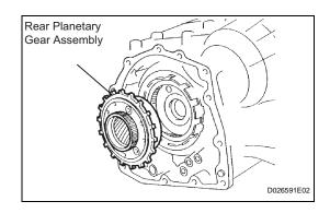
(b) Remove the rear planetary gear assembly from the transaxle case.
