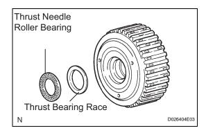
(b) Remove the thrust needle roller bearing and thrust bearing race from the rear planetary sun gear assembly.
