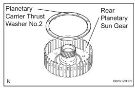
(c) Remove the planetary carrier thrust washer No.2 from the rear planetary sun gear assembly.
