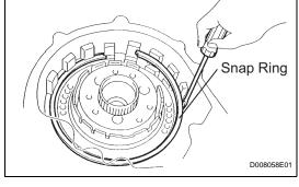
(b) Remove the 2ND brake piston assembly from the transaxle case.
