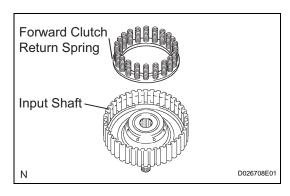
(d) Remove the forward clutch return spring from the input shaft.
