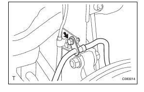
(b) Remove the 2 bolts and separate the rear disc brake caliper assembly.
