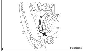
(c) Remove the bolt and the speed sensor front.
