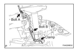
(b) Install the speed sensor front with the 2 bolts and the clamp.
