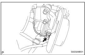
(b) Pull out the sensor wire harness with the with grommet.
