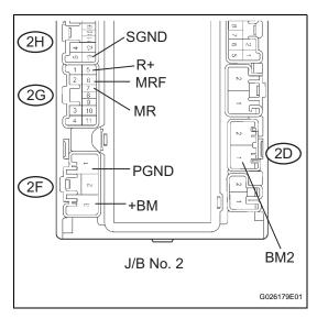
(b) Connect the battery positive lead to terminal +BM of the J/B No. 2 and the negative lead to terminal SGND, PGND, MRF and MR.
