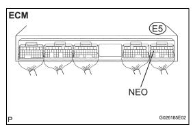
(a) Reconnect the ECM connector and the skid control ECU connector.
