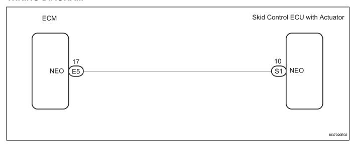
1 CHECK HARNESS AND CONNECTOR (SKID CONTROL ECU - ECM)
