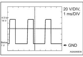
(b) Check the signal waveform between terminal NEO (E5-17) of the ECM and body ground for the engine conditions below.
