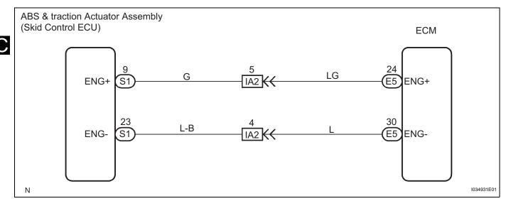
1 CHECK WIRE HARNESS AND CONNECTOR (ECM - SKID CONTROL ECU)
