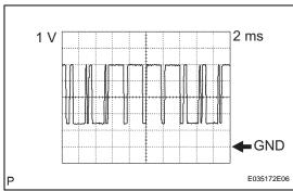
(d) Check the signal waveform between terminal LRDD (L1-3) of the laser sensor and body ground.
