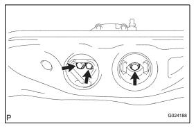
(c) Install the differential carrier assembly rear to the rear suspension member sub-assembly with the 3 bolts.
