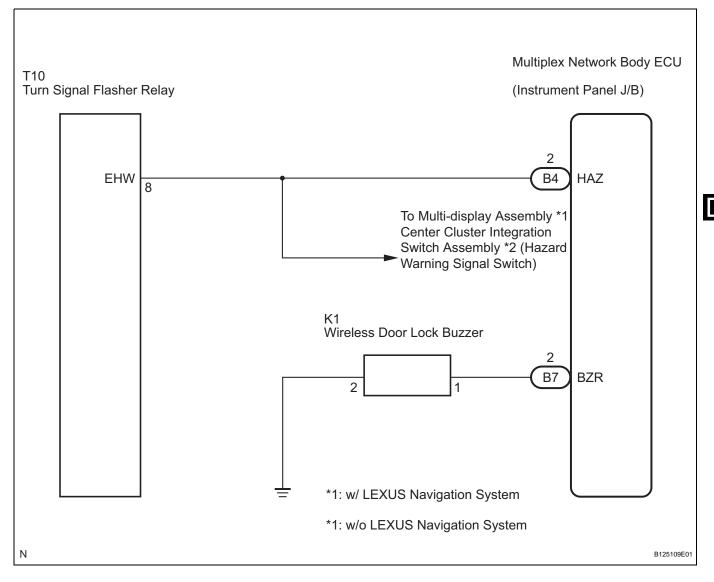
(a) Check that the wireless door lock functions operate when the transmitter is used (See page DL-63).
