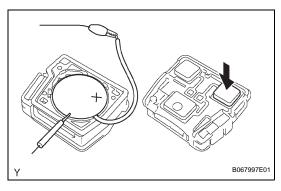
(2) Connect the lead to the negative (-) terminal of the transmitter and install the battery.
