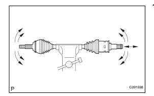
(h) Align the matchmarks, install the inboard joint assembly to the outboard joint shaft assembly.
