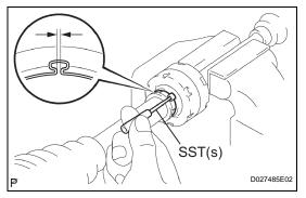
(e) Using SST(s), measure the clearance of the outboard joint boot No.2 clamp.
