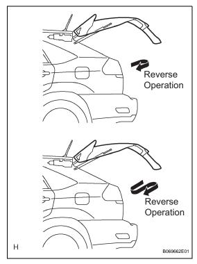
(3) While the back door is opening, press, by hand, the outside surface of the back door panel that is moving so that the operating speed decreases, as shown in the illustration.
