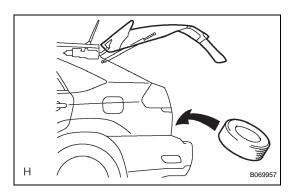
(4) [\*4] While the back door is closing, insert a tire or equivalent between the door panel and vehicle body, as shown in the illustration, in order to interrupt closing operation.
