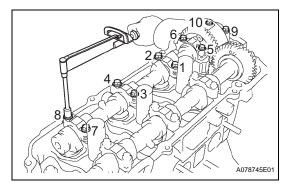
Using several steps, install and tighten the 10 bearing cap bolts uniformly in the sequence shown in the illustration.
