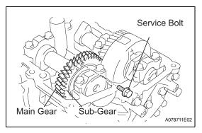
(b) Secure the exhaust camshaft sub-gear to the main gear with a service bolt.
