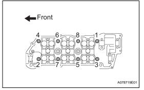
(e) Using several steps, loosen the 8 cylinder head bolts uniformly in the sequence shown in the illustration. Remove the 8 cylinder head bolts and plate washers.
