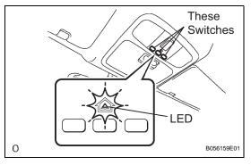
(b) Erase transmitter codes in the garage door opener clear mode. HINT:
