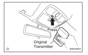
Press and hold the selected switch for 20 seconds. The garage door opener will enter registration mode. HINT:
